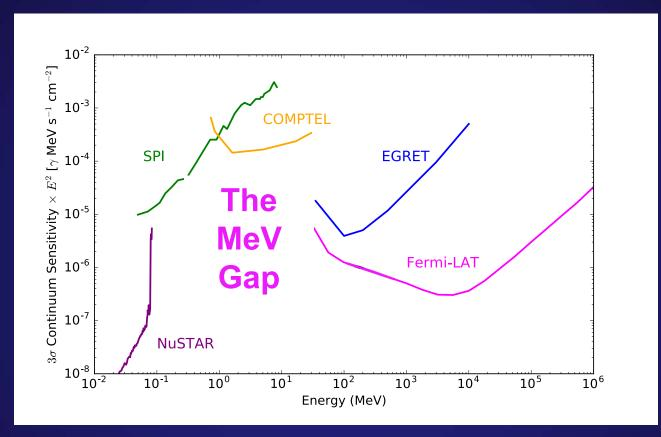
COMPTEL was the first, and still only, Compton Telescope to fly in space with sufficient sensitivity to perform astronomical observations in the MeV band
