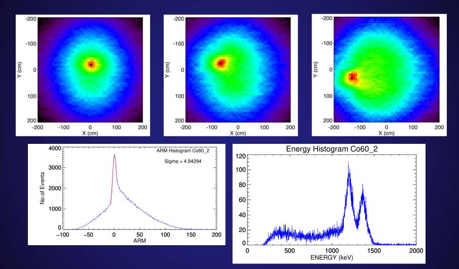
UNH energy calibration needs to be corrected using tagged source
