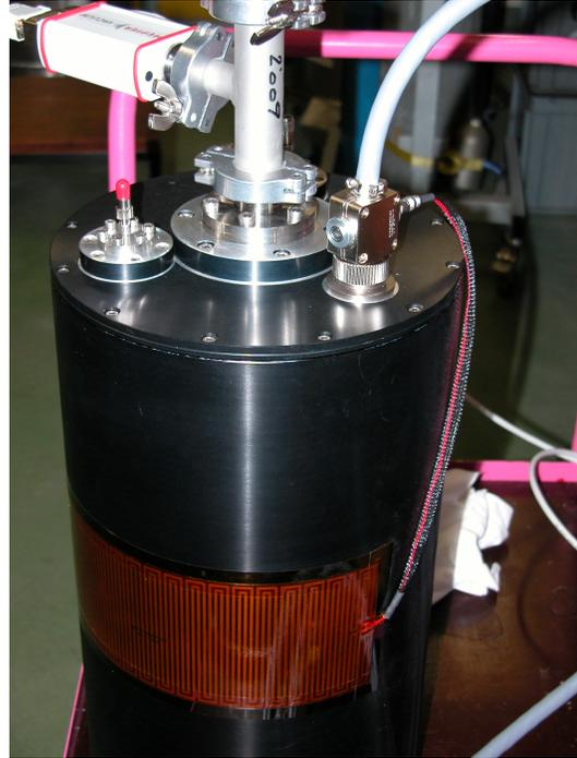
Fig 3: The FPCS in operation. The system is completely enclosed in the vacuum container. Light enters and exit the system via fiber optics feedthroughs. The heating pad seen on the bottom is part of the thermal control loop
