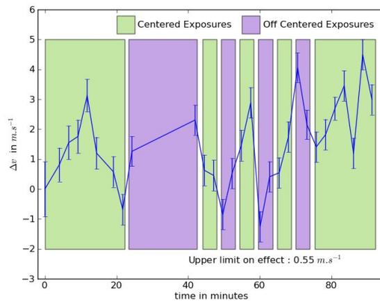
Figure 11: On sky test with HARPS-N: the star is observed, some exposure are made with the star centred (the purple zones) and other are off-centred (the star is on the border of the fiber). There is no obvious effect to be noted. An upper limit  $0.55 \text{ m s}^{-1}$  for the effect of decentring can be set. However this measure has not been done in an optimal way and the p-modes of the star are dominating all the effects.
