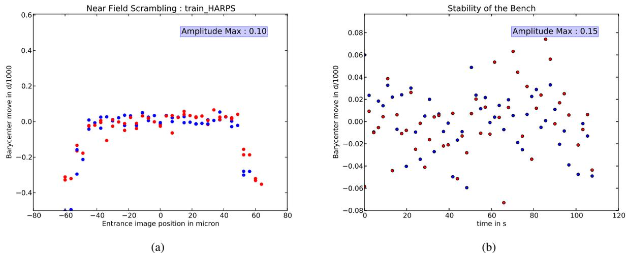
Figure 9: Illustration of the near field scrambling of the HARPS-N fiber train, in the laboratory. (a) the movements of the measurement in the near field of the scrambling performance of the whole fiber train. The scrambling Ratio is in the 10000 range. (b) limits of the measurement capability of the test bench. Red points are for the x axis on the CCD, blue points are for the y axis on the CCD. The orientation of these axes is arbitrary.
