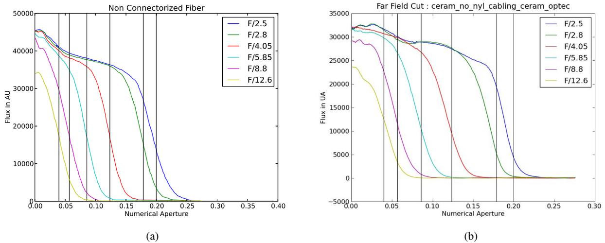
Figure 4: Profile of the far field of the octagonal fiber as a function of the entrance beam aperture. From these measurements one can calculate the FRD. (a) The naked fiber (b) The connectorized fiber.
