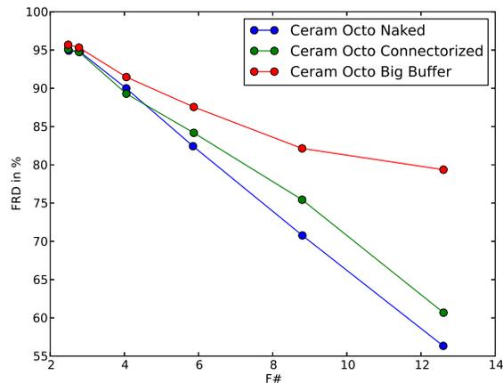
Figure 6: Compared FRD for 3 fibers: The octagonal fiber for HARPS-N, naked and connectorized and another octagonal fiber from the same company with a much larger cladding and buffer. The later has the best FRD we have ever measured. The fact that the naked fiber seems to have a worse FRD than the connectorized one is to be attributed to systematic errors in the measurements. One has to see they have a similar behaviour.
