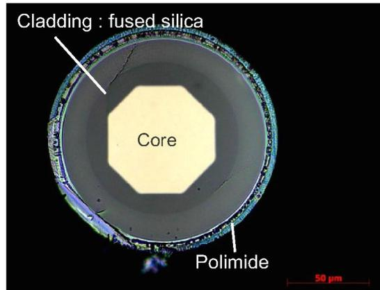
Figure 1: Photo of the manufactured fiber for HARPS-N
