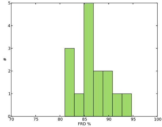
Figure 7: Histogram of all the measurement of the FRD measured at F/4 on all the ends of the fibre. All the fibers are better have an FRD better than 80%. The one used in the instrument have an FRD better than 85%.
