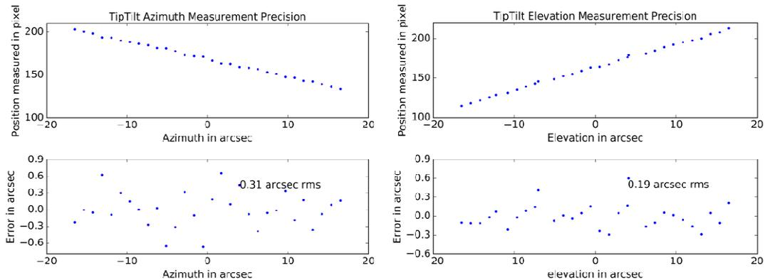
Figure 10 Graph showing the performance of the measurement of the tip-tilt using the dummy Payload CCD, these measurement have been performed in presence of the simulated jitter of the telescope. The PSF has been scanned using the Tip-Tilt mirror to produce these results. The achieved precision is around 0.3 arcsec
