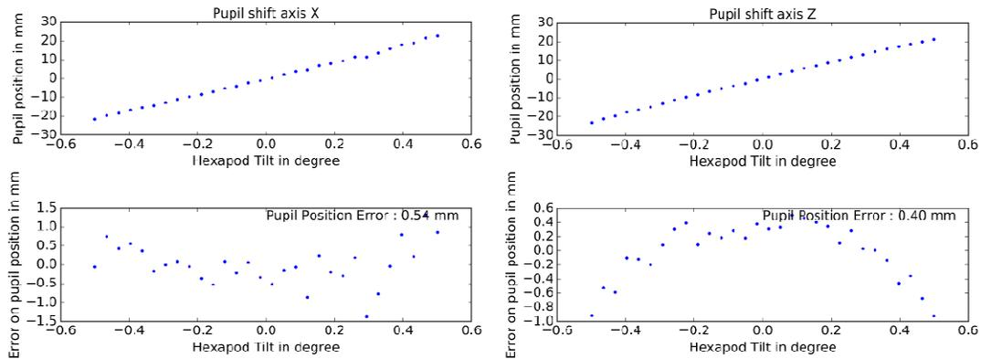
Figure 11 Graph showing the sensitivity of the pupil tracking measurement. The Hexapod below the focal plane is used to make the pupil scan across the pupil. The achievable precision is better than 0.5 mm/ over the 300 mm pupil which is fine to ensure the performances.
