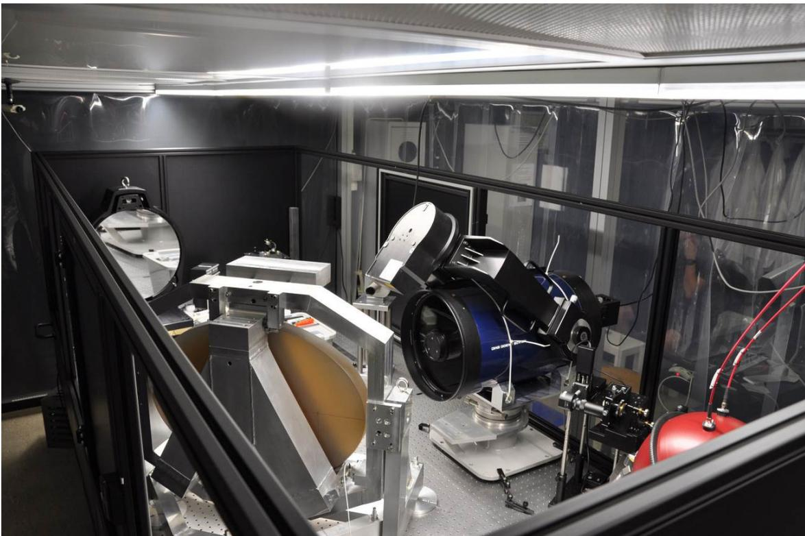
Figure 12. The CHEOPS calibration bench. The commercial telescope (in blue) simulates the CHEOPS payload. In operation the cover is fully closed
