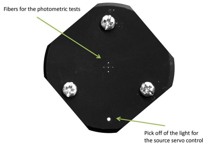
Figure 6. The picture shows the focal plane ferrule with the central star and the four fiducials. The dot at the bottom right is the fiber collecting the light from the pick-off mirror. The screws are holding the anti-reflection mask need to control ghosts.
