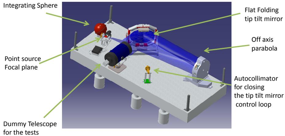
Figure 2. Side view of the calibration bench with the optical beam rendered in blue. This is the configuration used for the validation where a commercial telescope (in blue) simulates CHEOPS. The yellow device is a digital auto-collimator used to servo the folding flat in position.
