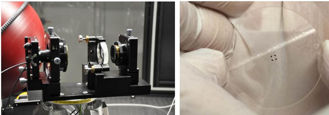
Figure 3. On the left, Side view of the focal plane module. On the right the mask, that allow for the masking of halves pupil on the 4 lateral sources.
