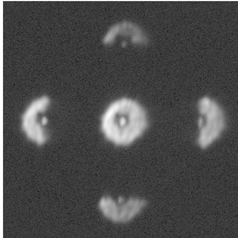
Figure 8 image of the focal plane in the star photometric mode. The central PSF is for the photometric measurement, while the 4 other PSFs are used to measure the pupil movements.
