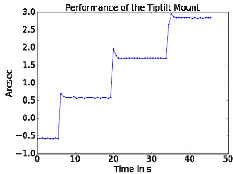
Figure 9 Performance of the tip tilt mount in its control loop mode
