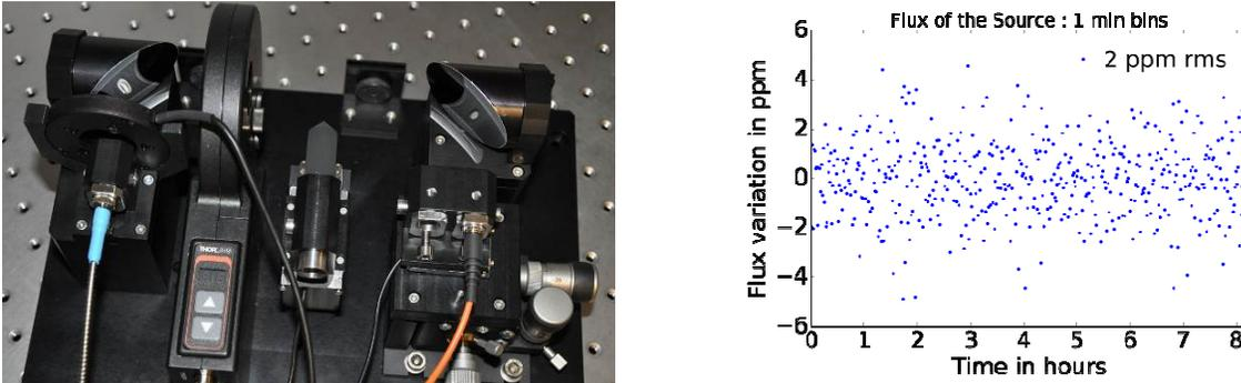
Figure 7. (Left) View of the super Stable source. (Right): performance of this source with stabilization. Stability is about 2ppm RMS when signal averaged in 1min bins
