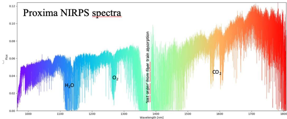
Figure 8. NIRPS spectra covers from 971 to 1854 nm over 70 spectral orders. One spectral order close to 1400 nm is lost due to the strong fiber OH absorption. The spectral resolution measured with the present grating is 82 000 in HA and 75 000 in HE. This data was obtained with a sub-optimal grating that has been replaced in July 2022 (see Section 7) and resolution should improve to >100 00 and >80 000 in HA and HE respectively.
