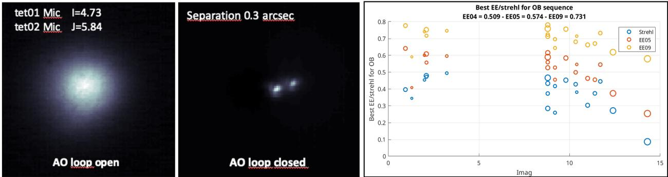
Figure 2. Illustration of the performances of the NIRPS AO system on Sky. (Left) Spatial resolution of the  $\theta$ Mic components. (Right) Strehl ratio and encircled energy in the HA and HE fibers as function of the star magnitude in the I band. More details can be found in [2].
