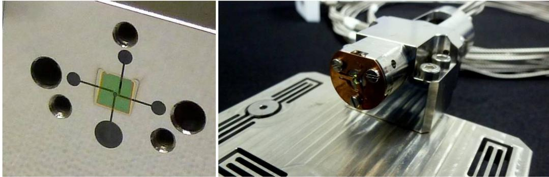
Figure 5. NIRPS Fiber Link Output End. (Left) The four fibers are closely packed together in a ferrule, at the end of the EDM generated slots. They are AR-coated (green square). (Right) The ferrule fitted with the adapting optics, mounted on the spectrograph interface plate.
