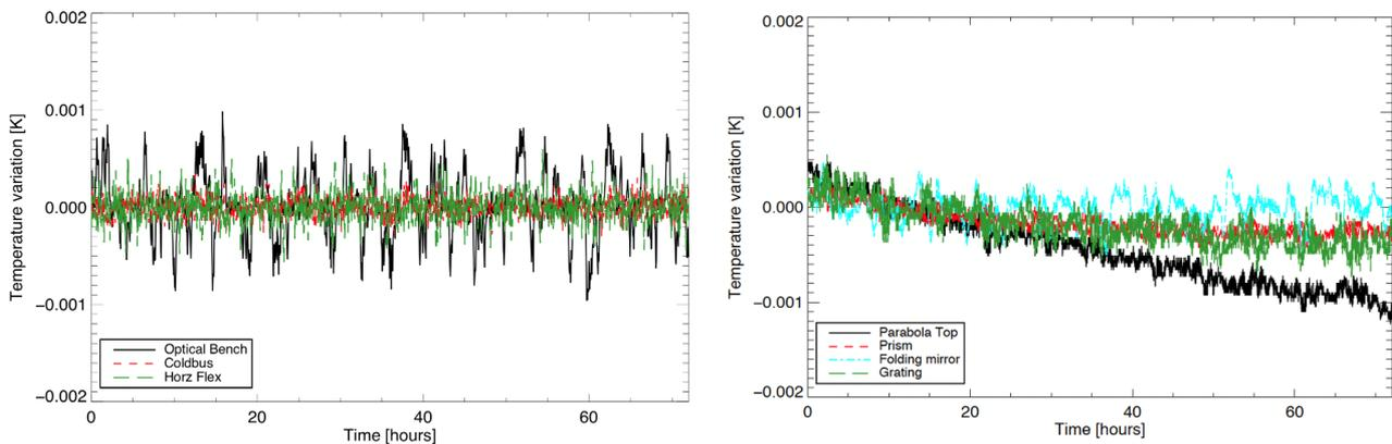
Figure 6. Temperature stability of the spectrograph cold bus. (Left) temperature measurements of various locations on the bench with active temperature regulation. (Right) temperature monitoring for some optical elements with no active temperature regulation. Overall, the temperature stability is at the sub-mK level over a period of three days.
