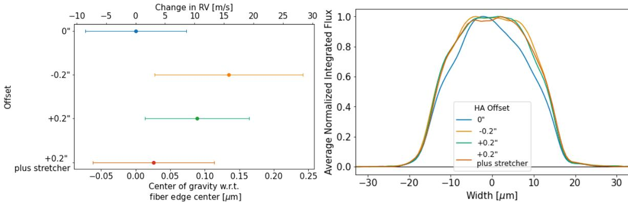
Figure 9. (Left) Relative variations of the measured RV as a function of PSF position on the tip of the fiber. Once activated, the stretcher resets the position-induced variation to almost 0. (Right) Normalized flux across the fiber tip. The smoothing effect of the stretcher is clearly visible
