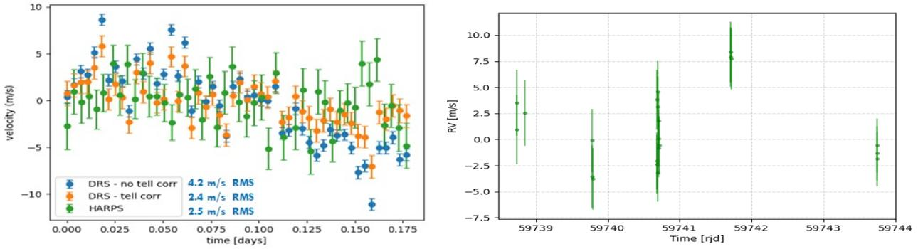
Figure 11. Preliminary raw results obtained during commissioning at the telescope using preliminary telluric correction and preliminary CCF masks. (Left) Proxima (M5V) over 4.2 hours showing RV precision < 3 m/s, slightly better than HARPS. (Right) Barnards star (M4V) over 6 nights showing RV precision of 3.3 m/s.
