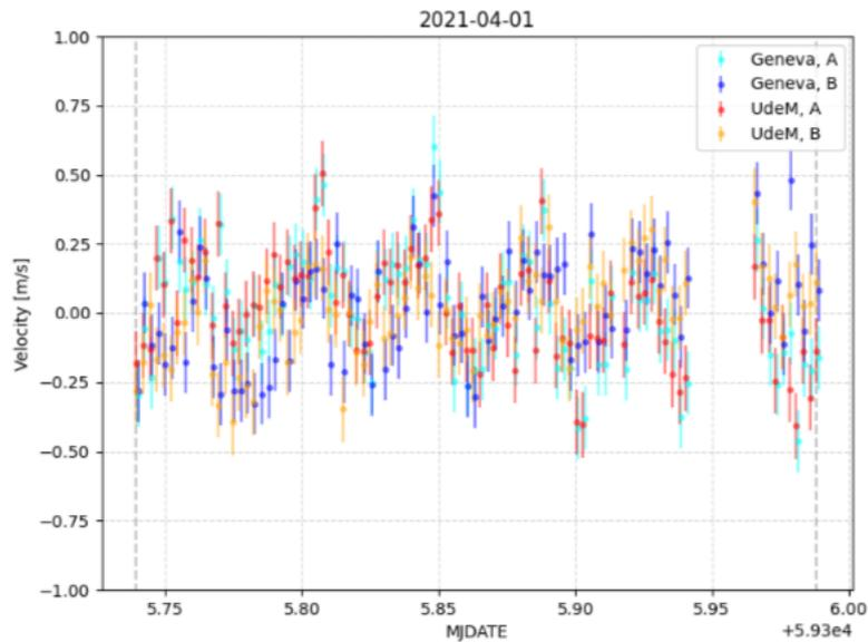
Figure 7. Intrinsic radial velocity stability of NIRPS measured in Lab on the HA mode showing a dispersion below 30 cm/s. The periodic modulations are correlated with room temperature.
