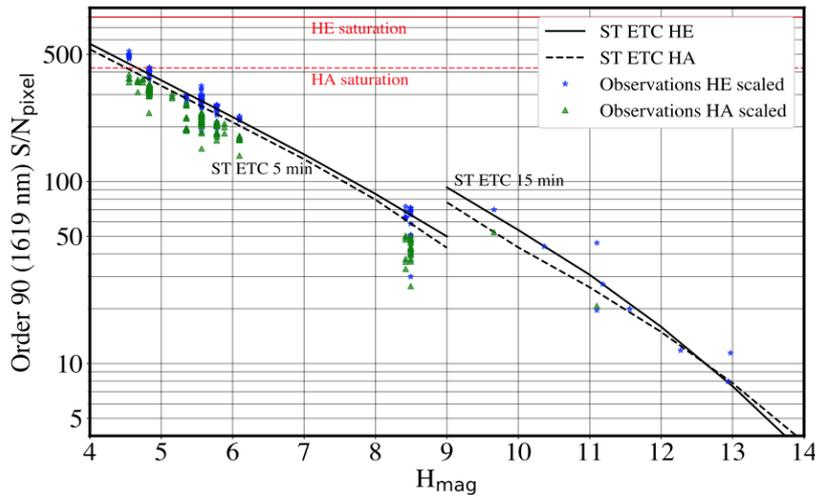
Figure 10. SNR computed at  $1.619 \mu\text{m}$  for all targets observed during commissioning with 5- and 15-min exposure time are in very good agreement with the expectation from the Science Team Exposure Time Calculator. Even slightly better than expected for HE mode. The limit magnitude of the AO system and guiding camera is  $I = 14.5$ .
