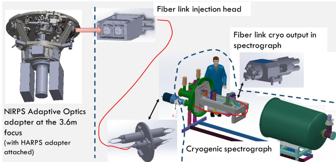
Figure 1. Overview of the NIRPS instrument.
