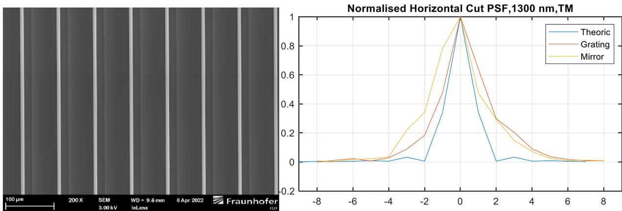
Figure 112. (Left) Micrograph of the etched silicon grating showing the exquisite quality of the grooves. (Right) PSF obtained on the grating test bench. There is no significant difference between the PSF obtained with the grating and the PSF obtained when replacing it with a plano mirror
