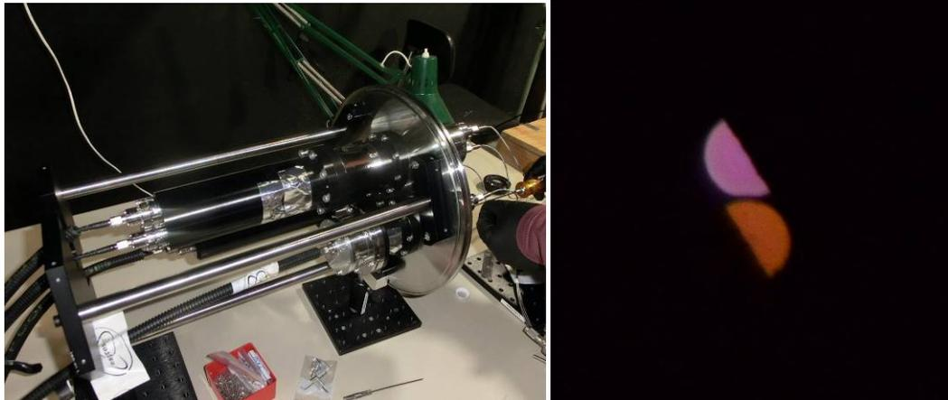
Figure 4. (Left) NIRPS Fiber Link Scrambler and (Right) an image of the pupil sliced
