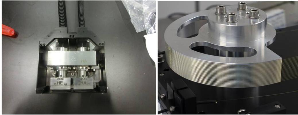
Figure 3. (Left): Fiber Link Input End on the Front End. (Right): The 20 loops of fiber coiled the stretcher half pulley.
