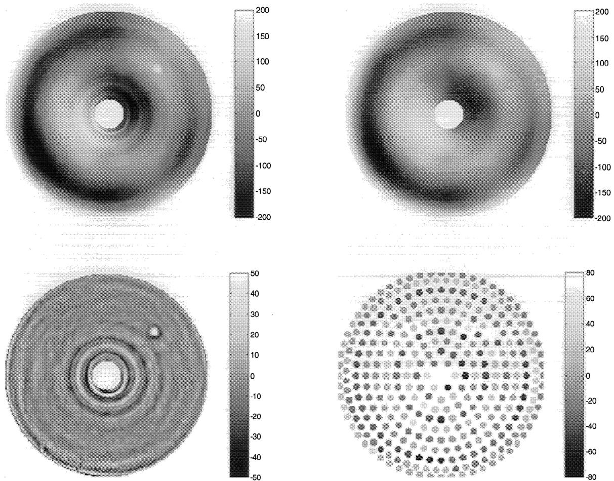
**Figure 4. Upper left: surface figure of the adaptive secondary shell bonded to the blocking body. Upper right: fit of actuator influence functions to the secondary figure. Lower left: residual error. Lower right: actuator forces that produce the best fit; the correction forces are the negative of these. Gray-level bars are labeled in nm of surface error for the surface maps, and mN for the actuator force diagram.**
