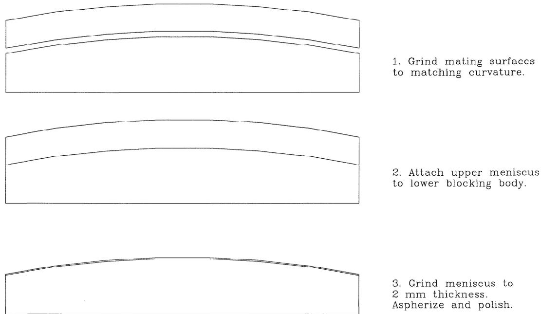
**Figure 1. Steps in the optical fabrication of the adaptive secondary shell.**
