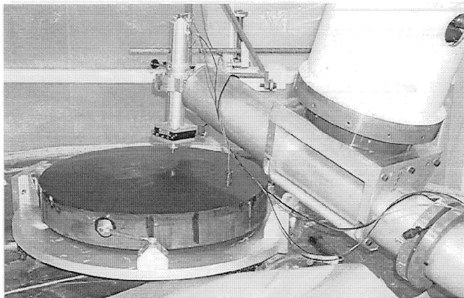
**Figure 3. Adaptive secondary shell, bonded to a rigid blocking body, being measured with the profilometer. The cylinder at upper right is the profilometer's bearing, aligned with the mirror's center of curvature.**
