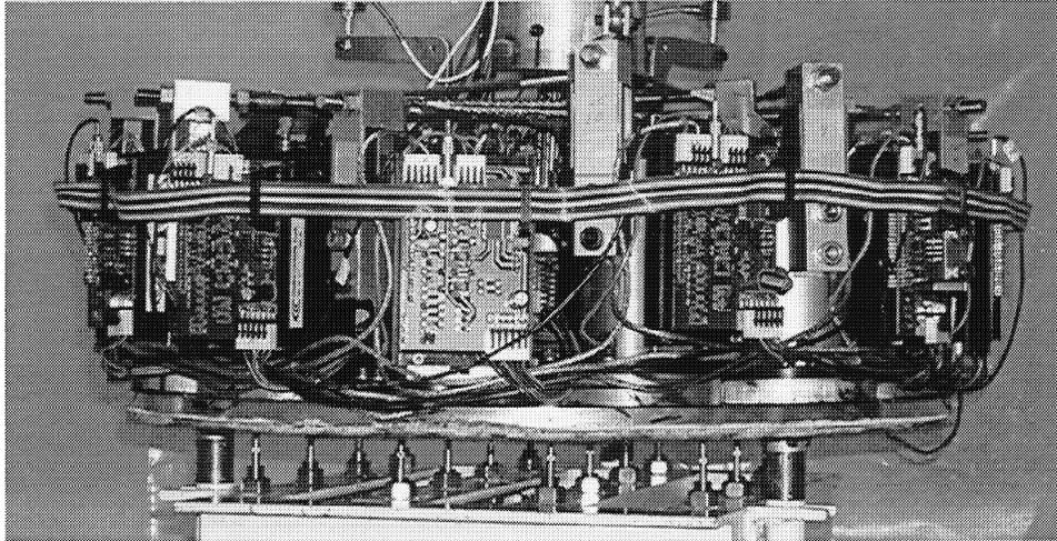
**Figure 2. Stressed lap used to figure the adaptive secondary mirror. The lap is mounted on an array of displacement sensors that measure its shape changes for testing and calibration. The lap's aluminum plate, 45 cm in diameter and 13 mm thick, is visible below the bending actuators. The plate is faced with pitch over a 30 cm diameter to form the polishing surface.**
